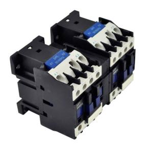
PART NUMBER – BLC2D0910-U7: BRAH Electric, aftermarket direct replacement reversing contactors for Telemecanique LC2D0910-U7, TeSys D Series, type LC2D, 3P, 3PH, 25A, 600V, 0.5-2HP @ 240V, 0.5-5HP @ 480V, 7.5HP @ 600V, both complete with 240V 50/60Hz AC coil, 1 N/O auxiliary contact, AC magnetic contactor, suitable for use with LC2-D series motor control systems
