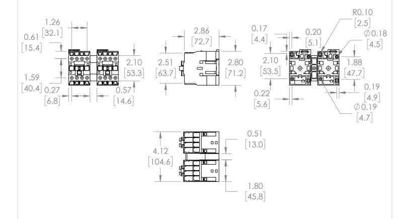
\*NOTE: BRAH ELECTRIC CONTACTOR BLC2D1210-B6 IS AN AFTERMARKET DIRECT REPLACMENT FOR LC2D1210-B6,LC2-D SERIES. SUITABLE FOR USE WITH LC2-D SERIES MOTOR CONTROL SYSTEMS
