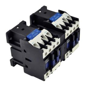
PART NUMBER – BLC2D1210-M6: BRAH Electric, aftermarket direct replacement contactors for Telemecanique LC2D1210-M6, TeSys D Series, direct substitute contactor, type LC2D, 3P, 3PH, 25A, 600V, 3HP @ 240V, 7.5HP @ 480V, 10HP @ 600V, complete with 220V AC coil, 1 N/O auxiliary contact, AC magnetic contactor suitable for use with LC2D series motor control systems
