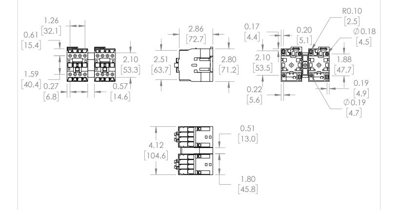
\*NOTE: BRAH ELECTRIC CONTACTOR BLC2D1210-R7 IS AN AFTERMARKET DIRECT REPLACMENT FOR LC2D1210-R7,LC2-D SERIES. SUITABLE FOR USE WITH LC2-D SERIES MOTOR CONTROL SYSTEMS
