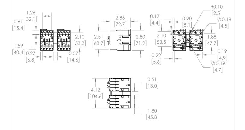
\*NOTE: BRAH ELECTRIC CONTACTOR BLC2D1210-U7 IS AN AFTERMARKET DIRECT REPLACMENT FOR LC2D1210-U7,LC2-D SERIES. SUITABLE FOR USE WITH LC2-D SERIES MOTOR CONTROL SYSTEMS
