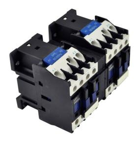
PART NUMBER – BLC2D2510-B6: BRAH Electric, aftermarket direct replacement reversing contactors for Telemecanique LC2D2510-B6, TeSys D Series, type LC2D, 3P, 3PH, 40A, 600V, 7.5HP @ 240V, 15HP @ 480V, 20HP @ 600V, both complete with 24V 60Hz AC coil, and 1 N/O auxiliary contact, AC magnetic contactor, suitable for use with LC2-D series motor control systems
