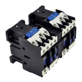
PART NUMBER – BLC2D2510-M6: BRAH Electric, aftermarket direct replacement reversing contactors for Telemecanique LC2D2510-M6, TeSys D Series, type LC2D, 3P, 3PH, 40A, 600V, 7.5HP @ 240V, 15HP @ 480V, 20HP @ 600V, both complete with 220V 60Hz AC coil, and 1 N/O auxiliary contact, AC magnetic contactor, suitable for use with LC2-D series motor control systems
