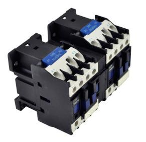
**PART NUMBER – BLC2D2510-T6**: BRAH Electric, aftermarket direct replacement reversing contactors for Telemecanique LC2D2510-T6, TeSys D Series, type LC2D, 3P, 3PH, 40A, 600V, 7.5HP @ 240V, 15HP @ 480V, 20HP @ 600V, both complete with 480V 60Hz AC coil, and 1 N/O auxiliary contact, AC magnetic contactor, suitable for use with LC2-D series motor control systems
