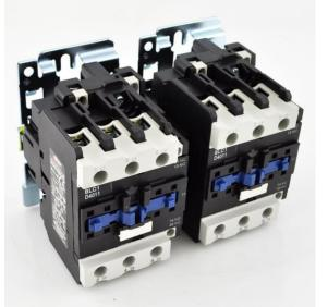
**PART NUMBER – BLC2D40**: BRAH Electric, aftermarket direct replacement reversing contactors for Telemecanique LC2D40, TeSys D Series, type LC2D, 3P, 3PH, 40A, 600V, 10HP @ 240V, 30HP @ 480V, 30HP @ 600V, both complete with 110/120V AC coil, and 1 N/O - 1 N/C auxiliary contact, AC magnetic contactor, suitable for use with LC2-D series motor control systems
