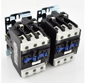
**PART NUMBER – BLC2D4011-T6**: BRAH Electric, aftermarket direct replacement reversing contactors for Telemecanique LC2D4011-T6, TeSys D Series, type LC2D, 3P, 3PH, 60A, 600V, 10HP @ 240V, 30HP @ 480V, 30HP @ 600V, both complete with 480V 60Hz AC coil, and 1 N/O - 1 N/C auxiliary contact, AC magnetic contactor, suitable for use with LC2-D series motor control systems
