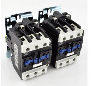
**PART NUMBER – BLC2D4011-U6:** BRAH Electric, aftermarket direct replacement reversing contactors for Telemecanique LC2D4011-U6, TeSys D Series, type LC2D, 3P, 3PH, 60A, 600V, 10HP @ 240V, 30HP @ 480V, 30HP @ 600V, both complete with 240V 60Hz AC coil, and 1 N/O - 1 N/C auxiliary contact, AC magnetic contactor, suitable for use with LC2-D series motor control systems
