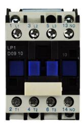
PART NUMBER – BLP1D09: BRAH Electric, aftermarket direct replacement reversing contactors for Telemecanique LP1D09, TeSys D Series, type LP1, 3P, 3PH, 9A, 600V, 2HP @ 240V, 5HP @ 480V, 7.5HP @ 600V, complete with 120V DC coil, 1 N/O auxiliary contact, DC magnetic contactor, suitable for use with
