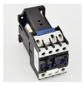
PART NUMBER – BLP1D2510BD: BRAH Electric, aftermarket direct replacement contactors for Telemecanique LP1D2510BD, TeSys D Series, type LP1D, 3P, 3PH, 40A, 600V, 7.5HP @ 240V, 15HP @ 480V, 20HP @ 600V, complete with 24V DC coil, 1 N/O auxiliary contact, DC magnetic contactor, suitable for use with LP1-D series motor control systems
