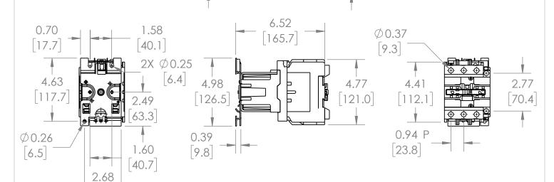
\*NOTE: BRAH ELECTRIC CONTACTOR BLP1D6510BD IS AN AFTERMARKET DIRECT REPLACMENT FOR LP1D6510BD,LP1-D SERIES. SUITABLE FOR USE WITH LP1-D SERIES MOTOR CONTROL **SYSTEMS**
