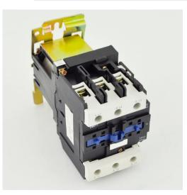
PART NUMBER – BLP1D8010GD: BRAH Electric, aftermarket direct replacement contactors for Telemecanique LP1D8010GD, TeSys D Series, type LP1D, 3P, 3PH, 125A, 600V, 30HP @ 240V, 60HP @ 480V, 60HP @ 600V, complete with 120V DC coil, 1 N/O auxiliary contact, DC magnetic contactor, suitable for use with LP1-D series motor control systems
