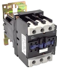
PART NUMBER – BLP1D9510UD: BRAH Electric, aftermarket direct replacement contactors for Telemecanique LP1D9510UD, TeSys D, type LP1D, 3P, 3PH, 125A, 600V, 30HP @ 240V, 60HP @ 480V, 60HP @ 600V, complete with 250V DC coil, 1 N/O auxiliary contact, DC magnetic contactor, suitable for use with LP1-D series motor control systems
