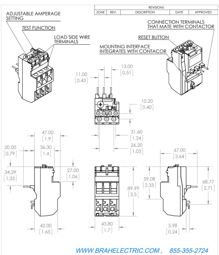
\*NOTE: BRAH ELECTRIC OVERLOAD RELAY BLR2D1301 IS AN AFTERMARKET DIRECT REPLACEMENT FOR LR2D1301, LR2D SERIES. SUITABLE FOR USE WITH LR2D SERIES MOTOR CONTROL SYSTEMS.
