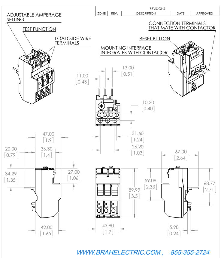
\*NOTE: BRAH ELECTRIC OVERLOAD RELAY BLR2D1303 IS AN AFTERMARKET DIRECT REPLACEMENT FOR LR2D1303, LR2D SERIES. SUITABLE FOR USE WITH LR2D SERIES MOTOR CONTROL SYSTEMS.
