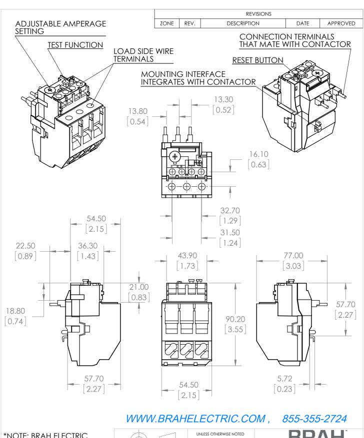
\*NOTE: BRAH ELECTRIC OVERLOAD RELAY BLR2D2355 IS AN AFTERMARKET DIRECT REPLACEMENT FOR LR2D2355, LR2D SERIES. SUITABLE FOR USE WITH LR2D SERIES MOTOR CONTROL SYSTEMS.
