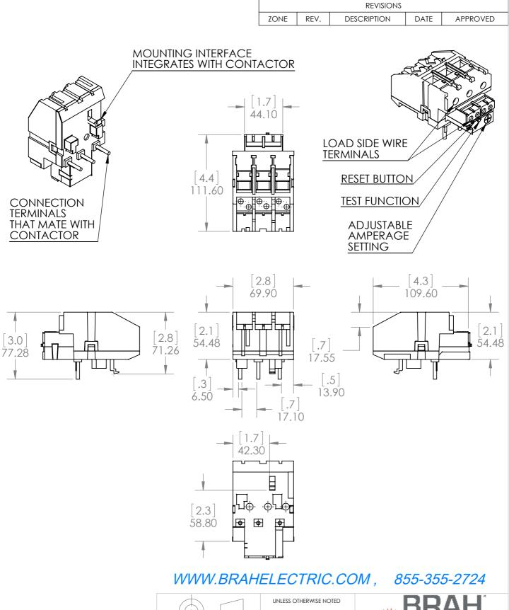
\*NOTE: BRAH ELECTRIC **OVERLOAD RELAY** BLR2D3355 AN AFTERMARKET DIRECT REPLACMENT FOR LR2D3355.SUITABLEFOR USE WITH LC1D AND LC2D **CONTACTORS**
