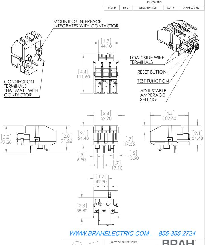
\*NOTE: BRAH ELECTRIC **OVERLOAD RELAY** BLR2D3357 AN AFTERMARKET DIRECT REPLACMENT FOR LR2D3357.SUITABLE FOR USE WITH LC1D AND LC2D **CONTACTORS**
