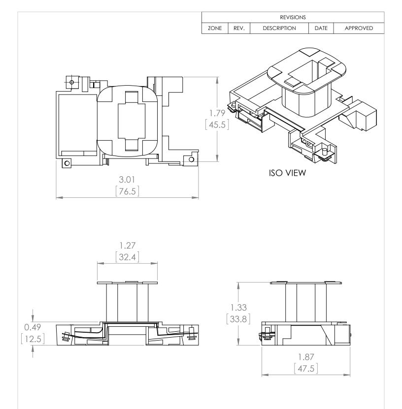
\*NOTE: BRAH ELECTRIC COILS BLX1D4B6 ARE A DIRECT REPLACEMENT FOR TELEMECANIQUE LX1D4B6, TESYS D SERIES, SUITABLE FOR USE WITH LC1D25, LC1D32, LC2D25, LC2D32 CONTACTORS
