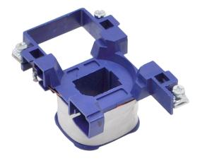
**PART NUMBER - BLX1D4M7 :** BRAH Electric, aftermarket direct replacement coils for Telemecanique LX1D4M7, TeSys D Series, type BLX1D, 220V AC 50/60Hz, suitable for use with LC1D25, LC1D32, LC2D25, LC2D32 contactors
