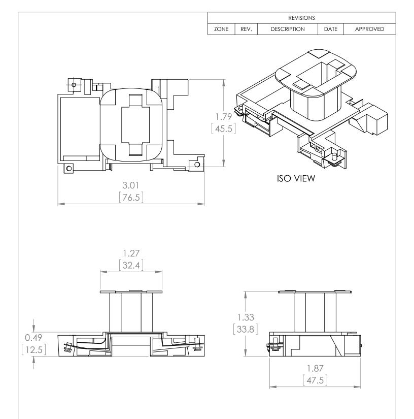
\*NOTE: BRAH ELECTRIC COILS BLX1D4U7 IS A DIRECT REPLACEMENT FOR TELEMECANIQUE LX1D4U7, TESYS D SERIES, SUITABLE FOR USE WITH LC1D25, LC1D32, LC2D25, LC2D32 CONTACTORS
