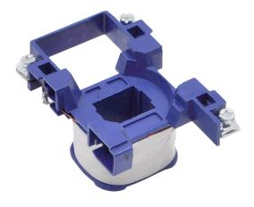
**PART NUMBER - BLX1D4W6:** BRAH Electric, aftermarket direct replacement coils for Telemecanique LX1D4W6, TeSys D Series, type BLX1D, 277V AC 60Hz, suitable for use with LC1-D, 25 and 32 amp contactors
