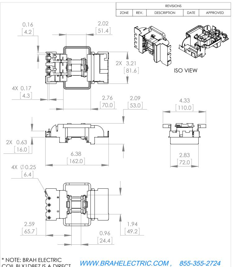
COIL BLX1D8E7 IS A DIRECT REPLACEMENT FOR TELEMECANIQUE LX1D8E7, TESYS D SERIES, SUITABLE FOR USE WITH ALL 3P AND 4P LC1D115, LC1D150, LC2D115, LC2D150 CONTACTORS
