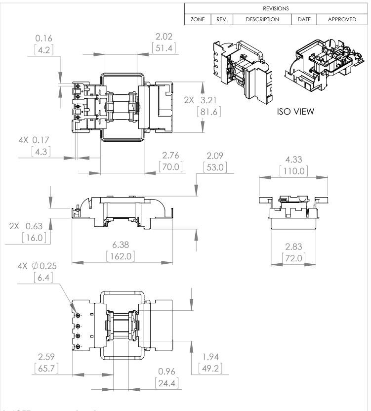
\* NOTE: BRAH ELECTRIC COIL BLX1D8M7 IS A DIRECT REPLACEMENT FOR **TELEMECANIQUE** LX1D8M7, TESYS D SERIES, SUITABLE FOR USE WITH ALL 3P AND 4P LC1D115, LC1D150, LC2D115, LC2D150 CONTACTORS
