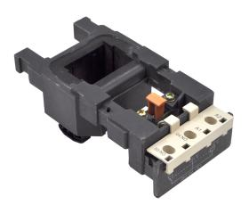
**PART NUMBER - BLX1FG162:** BRAH Electric, aftermarket direct replacement coils for Telemecanique LX1FG162, TeSys F Series, type BLX1F, 200/208VAC 60Hz, coil suffix code is L6, suitable for use with all 3P and 4P LC1F185, LC1F225, LC2F185, LC2F225 contactors
