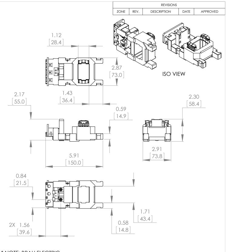
\* NOTE: BRAH ELECTRIC COIL BLX1FG380 IS A DIRECT REPLACEMENT FOR TELEMECANIQUE LX1FG380, TESYS F SERIES, SUITABLE FOR USE WITH ALL 3P AND 4P LC1F185, LC1F225, LC2F185, LC2F225 CONTACTORS
