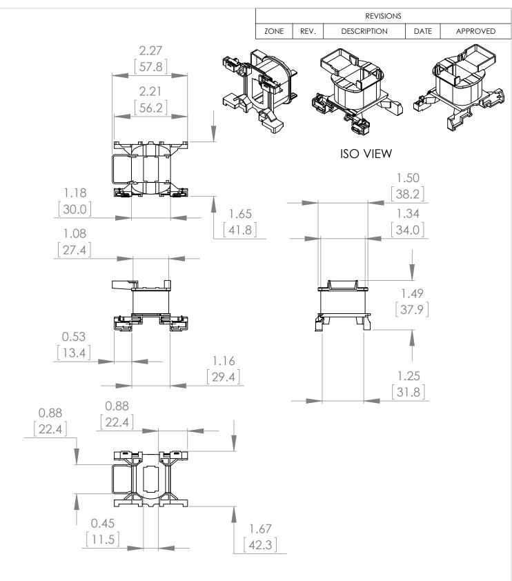
\* NOTE: BRAH ELECTRIC COIL BLXD1B6 IS A DIRECT REPLACEMENT FOR TELEMECANIQUE LXD1B6, TESYS D SERIES, SUITABLE FOR USE WITH 3P AND 4P LC1D09, LC1D12, LC1D18, LC2D09, LC2D12, LC2D18, LC1DT20, LC1DT40 CONTACTORS
