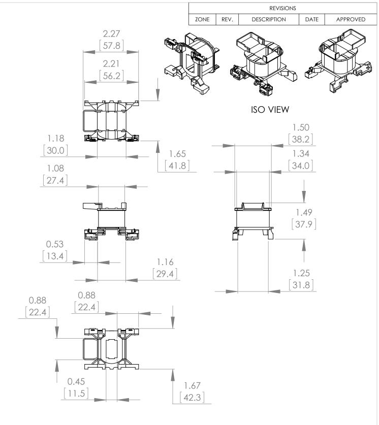
\* NOTE: BRAH ELECTRIC COIL BLXD1M6 IS A DIRECT REPLACEMENT FOR TELEMECANIQUE LXD1M6, TESYS D SERIES, SUITABLE FOR USE WITH 3P AND 4P LC1D09, LC1D12, LC1D18, LC2D09, LC2D12, LC2D18, LC1DT20, LC1DT40 CONTACTORS
