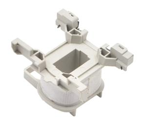
PART NUMBER - BLXD1M6: BRAH Electric, aftermarket direct replacement coils for Telemecanique LXD1M6, TeSys D Series, type BLXD1, 220VAC 60Hz, suitable for use with 3P and 4P LC1D09, LC1D12, LC1D18, LC2D09, LC2D12, LC2D18, LC1DT20, LC1DT40 contactors
