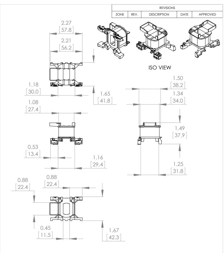
\* NOTE: BRAH ELECTRIC COIL **BLXD1U7 IS A DIRECT** REPLACEMENT FOR TELEMECANIQUE LXD1U7, TESYS D SERIES, SUITABLE FOR USE WITH 3P AND 4P LC1D09, LC1D12, LC1D18, LC2D09, LC2D12, LC2D18, LC1DT20, LC1DT40 CONTACTORS
