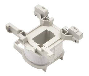
**PART NUMBER - BLXD1U7:** BRAH Electric, aftermarket direct replacement coils for Telemecanique LXD1U7, TeSys D Series, type BLXD1, 240VAC 50/60Hz, suitable for use with 3P and 4P LC1D09, LC1D12, LC1D18, LC2D09, LC2D12, LC2D18, LC1DT20, LC1DT40 contactors
