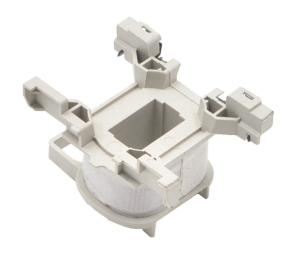
**PART NUMBER - BLXD1W7:** BRAH Electric, aftermarket direct replacement coils for Telemecanique LXD1W7, TeSys D Series, type BLXD1, 277VAC 50/60Hz, suitable for use with 3P and 4P LC1D09, LC1D12, LC1D18, LC2D09, LC2D12, LC2D18, LC1DT20, LC1DT40 contactors
