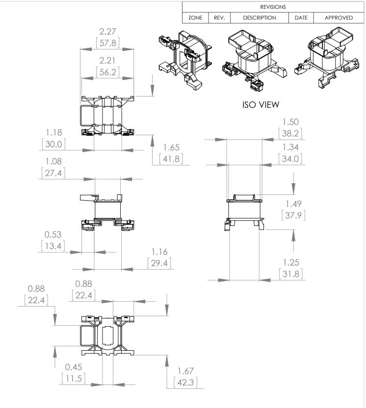
\* NOTE: BRAH ELECTRIC COIL BLXD1W7 IS A DIRECT REPLACEMENT FOR TELEMECANIQUE LXD1W7, TESYS D SERIES, SUITABLE FOR USE WITH 3P AND 4P LC1D09, LC1D12, LC1D18, LC2D09, LC2D12, LC2D18, LC1DT20, LC1DT40 CONTACTORS
