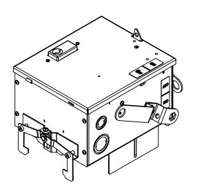
\* NOTE: BRAH Electric aftermarket direct RV421, 30amp, 240volt, 3 phase, 4 wire, fusible style bus plug, type BRV/RV, Suitable for use with OEM ITE/ siemens XL-X series industrial Busway System.
