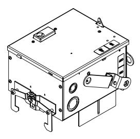
\* NOTE: BRAH Electric aftermarket direct,30amp, 240volt, 3 phase, 3 wire, fusible style bus plug, type BRV/RV, Suitable for use with OEM ITE/ siemens XL-X series industrial Busway System. FROPRIETARY AN DRAWING IS THE SI BRAH ELECTRIC. A IN PART OR AS A W WRITEN PERMISSIO IS PROHIBITED.
