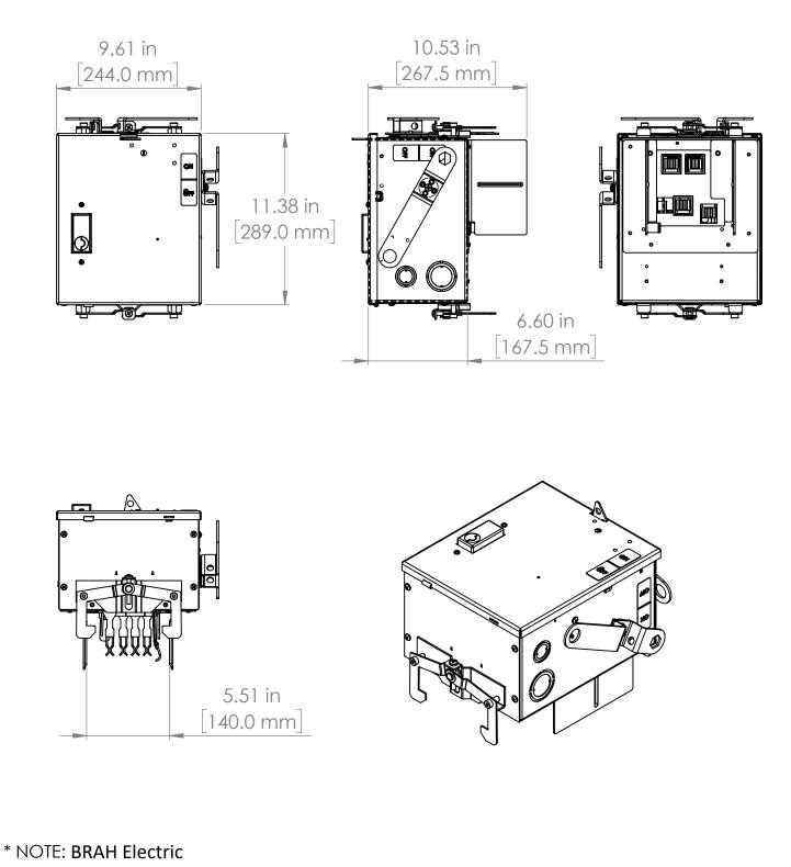
aftermarket direct, 30amp, 600volt, 3 phase, 3 wire, fusible style bus plug, type BRV/RV, Suitable for use with OEM ITE/ siemens XL-X series industrial Busway System.
