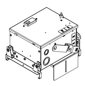
\* NOTE: BRAH Electric aftermarketdirect UV462G, 60amp, 600volt, 3 phase, 4 wire, fusible style bus plug, type BUV / UV, suitable for use with OEM ITE/ siemens XL-U series Industrial Busway Systems.
