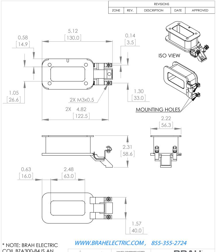
\* NOTE: BRAH ELECTRIC COIL BZA300-84 IS AN AFTERMARKET DIRECT REPLACEMENT FOR ABB ZA300-84, A-LINE SERIES, SUITABLE FOR USE WITH A210, A260, A300 CONTACTORS
