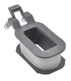
**PART NUMBER - BZA300-86:** BRAH Electric, aftermarket direct replacement coils for ABB ZA300-86, A-Line Series, type BZA, 440V AC 60Hz, suitable for use with A210, A260, A300 contactors
