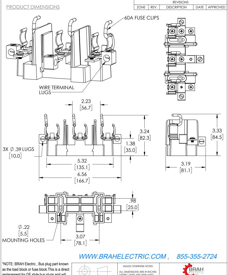
replacement for GE style bus plugs and will fit All Spectra series, Spectra low amp, Armor Clad and Flex-A plug Bus Plugs, substitute for OEM General Electric, engineered to operate on 240 volt systems, 3 phase, 240 volt, 60 amp maximum.
