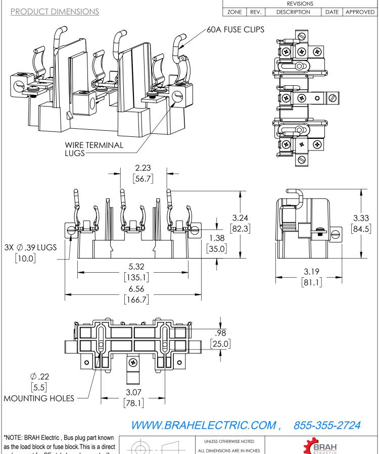
replacement for GE style bus plugs and will fit All Spectra series, Spectra low amp, Armor Clad and Flex-A plug Bus Plugs, substitute for OEM General Electric, engineered to operate on both 240 volt and 600 volt systems, 3 phase, 600 volt, 60 amp maximum.
