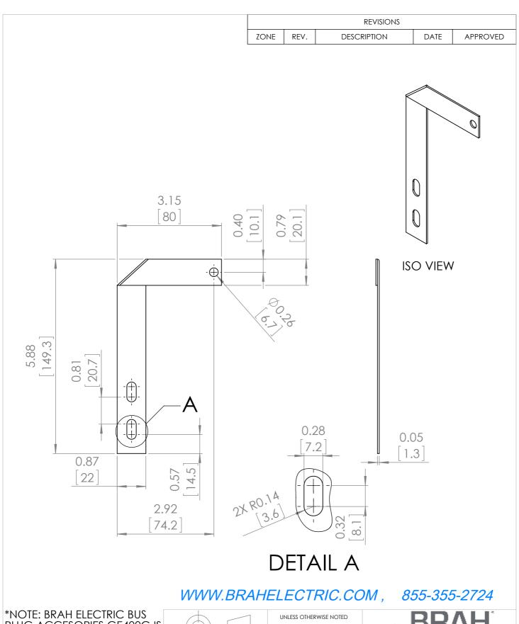
PLUG ACCESORIES GE400G IS AN AFTERMARKET DIRECT REPLACEMENT FOR GENERAL ELECTRIC, SPECTRA SERIES, GROUND KITS, GROUND KIT ASSEMBLIES, 400-600A, TO BE USED WITH TYPE AC, SB, SL BUS PLUGS
