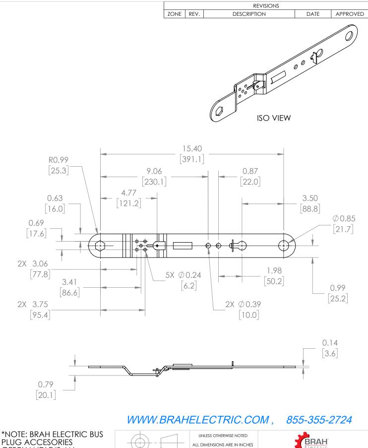
GEBPHANDLE IS AN AFTERMARKET DIRECT REPLACMENT, SUITABLE FOR USE WITH AC, SB, SL, FVK BREAKER TYPE AND FUSIBLE **BUS PLUGS**
