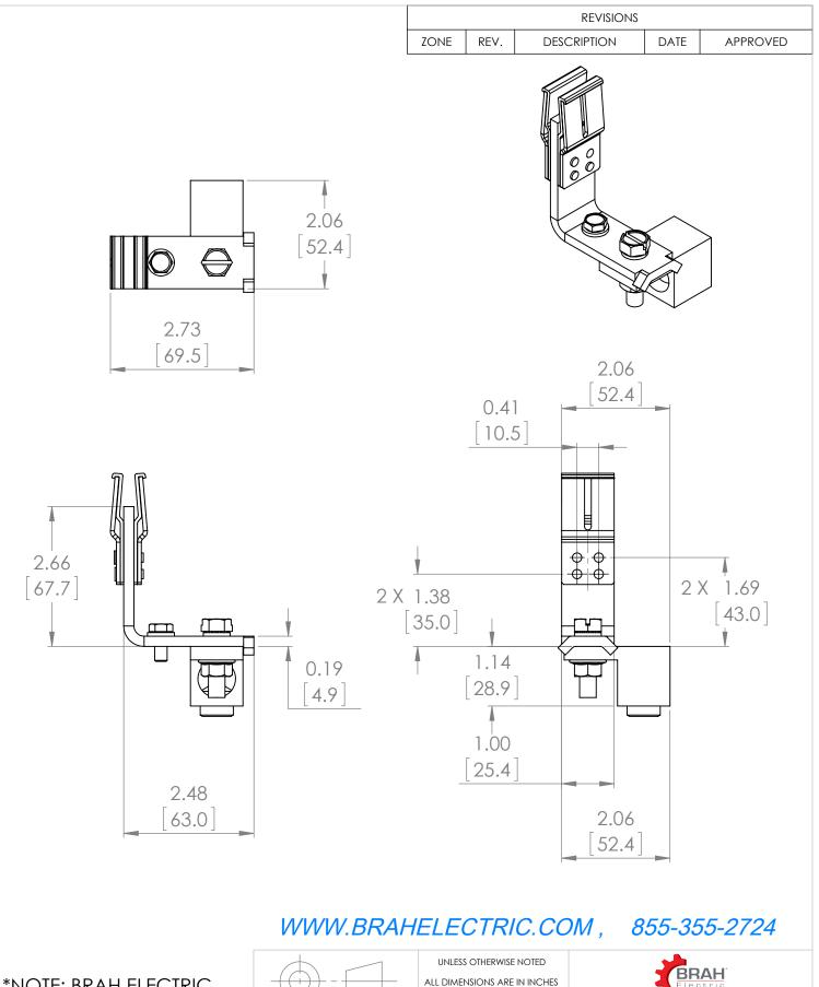
\*NOTE: BRAH ELECTRIC DIRECT REPLACEMENT **NEUTRAL KITS FOR** SQUARE D, I-LINE, 600V, 250A, SUITABLE FOR USÉ WITH 250A PKA, PKH, PKC FRAME I-LINE BUS PLUGS THIRD ANGLE PROJECTION
