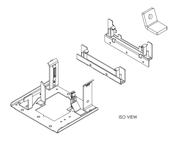
\* NOTE: BRAH ELECTRIC CONVERSION KITS ARE A DIRECT REPLACEMENT FOR GENERAL ELECTRIC, SPECTRA LOW-AMP SERIES, TYPE ACSL, 600V MAX, WITH GROUND, FOR USE WITH 110A-250A RATED BUS PLUGS.
