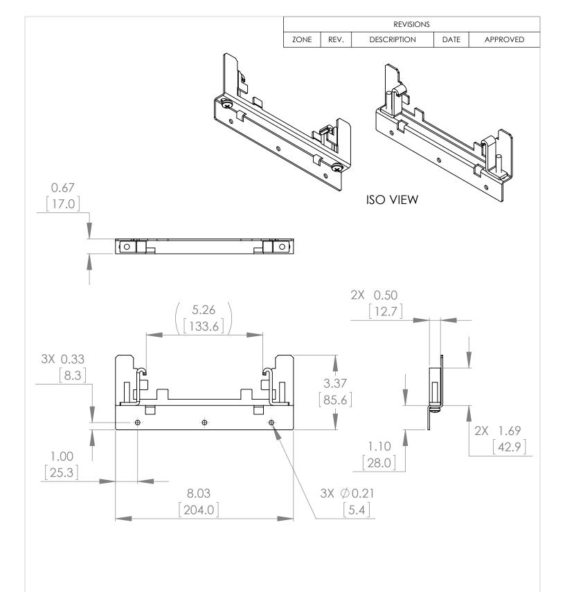
\* NOTE: BRAH ELECTRIC CONVERSION KITS ARE A DIRECT REPLACEMENT FOR GENERAL ELECTRIC, SPECTRA LOW-AMP SERIES, TYPE ACSL, 600V MAX, WITH GROUND, FOR USE WITH 110A-250A RATED BUS PLUGS.
