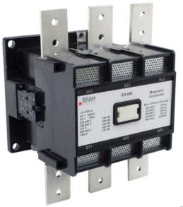
PART NUMBER - BEH-800-30-22: BRAH Electric, aftermarket direct replacement contactors for ABB EH-800-30-22, EH Series, type EH, 3P, 3PH, 750A, 600V, 300HP @ 240V, 600HP @ 480V, 700HP @ 600V, complete with 120V AC coil, 2 N/O - 2 N/C auxiliary contact, AC magnetic contactor, suitable for use with EH series motor control systems
