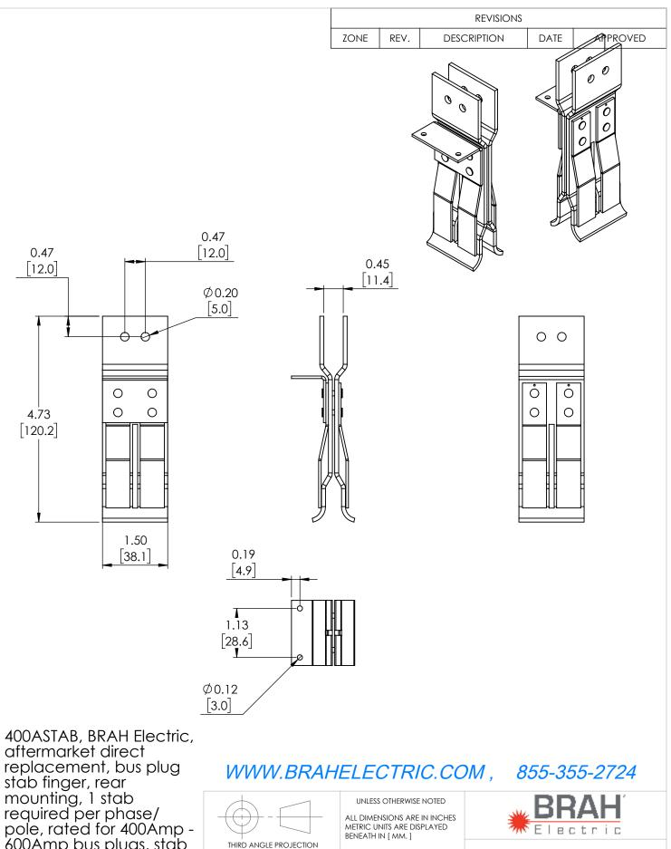
600Amp bus plugs, stab suitable for use with GE Armor Clad, Spectra SB, and Spectra Low-Amp SL bus plugs
