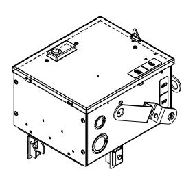
\* NOTE: BRAH Electric aftermarket direct ITAP322G,60amp, 240volt, 3 phase, 3 wire, fusible style bus plug,type BIP/ITAP, suitable for use with OEM Westinghouse /Cutler hammer/Eaton POW-R-WAY I & II Industrial Busway System.
