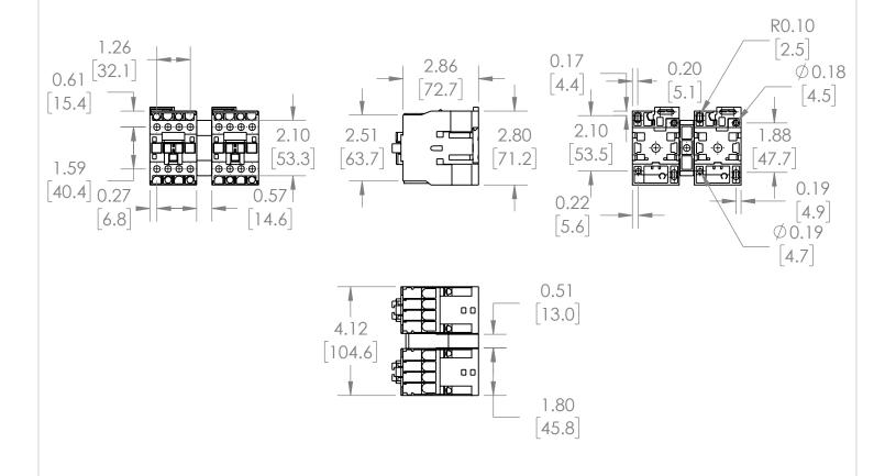
\*NOTE: BRAH ELECTRIC CONTACTOR BLC2D18 IS AN AFTERMARKET DIRECT REPLACMENT FOR LC2D18, LC2-D SERIES. SUITABLE FOR USE WITH LC2-D SERIES MOTOR CONTROL SYSTEMS
