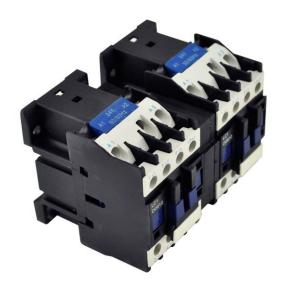
PART NUMBER – BLC2D1810: BRAH Electric, aftermarket direct replacement contactors for Telemecanique LC2D1810, TeSys D, direct substitute contactor, type LC2D, 3P, 3PH, 32A, 600V, 5HP @ 240V, 10HP @ 480V, 15HP @ 600V, complete with 110/120V AC coil, 1 N/O auxiliary contact, AC magnetic contactor suitable for use with LC2D series motor control systems
